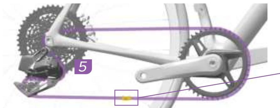
Pull each end of the chain together and install the PLCK-D1 PowerLock. Press the PowerLock connector links together.
