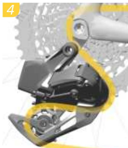
Place the chain onto the smallest cassette cog. Route the chain through the rear derailleur pulleys, and above the tab in the cage.
