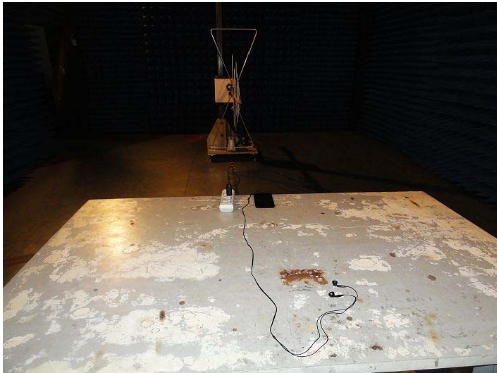
Radiated Emission Test Setup:
