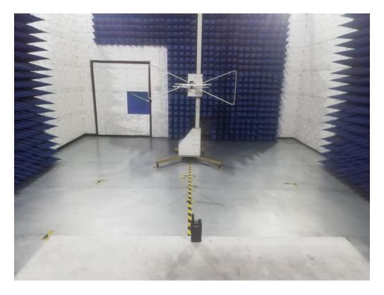
RADIATED EMISSION ABOVE 1G TEST SETUP
