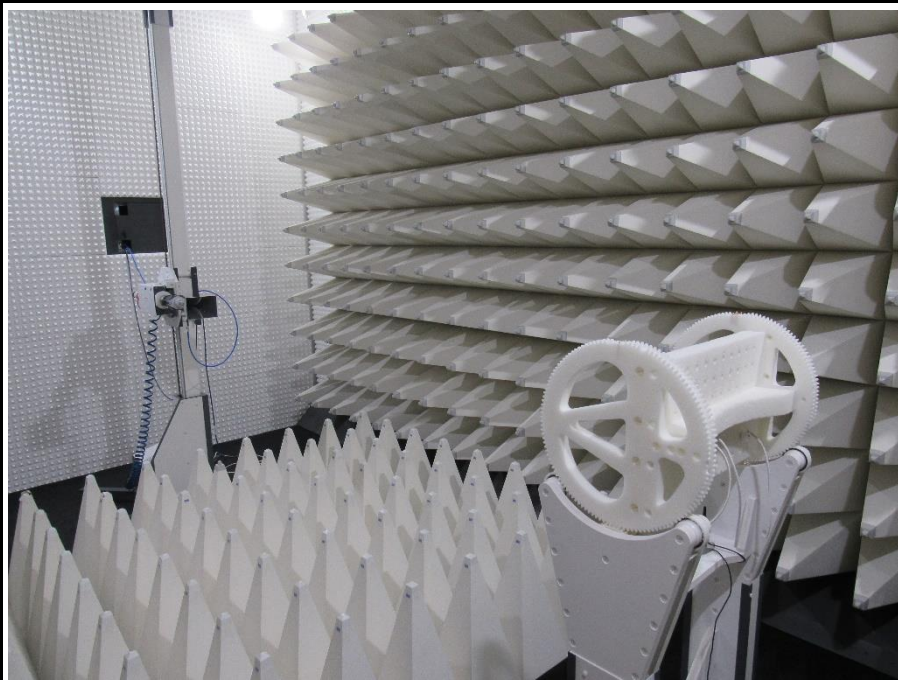
Setup for measurements above 1 GHz
