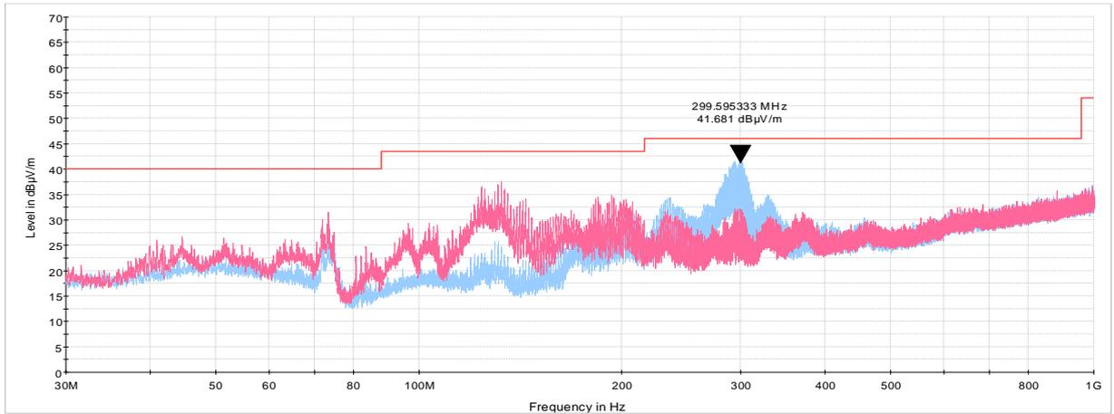
**Plot 7.2.11 Radiated emission measurements from 30 to 1000 MHz at the mid carrier frequency**
