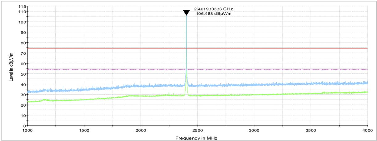
**Plot 7.2.14 Radiated emission measurements from 1 to 4 GHz at the mid carrier frequency**
