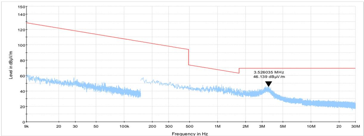
**Plot 7.2.8 Radiated emission measurements from 9 kHz to 30 MHz at the mid carrier frequency**
