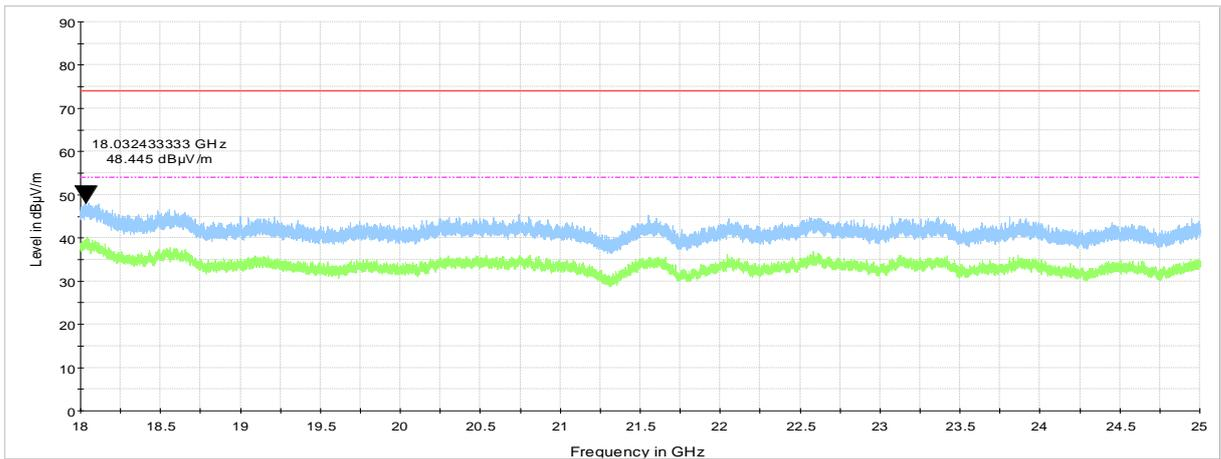
**Plot 7.2.20 Radiated emission measurements from 18 GHz to 25 GHz at the mid carrier frequency**
