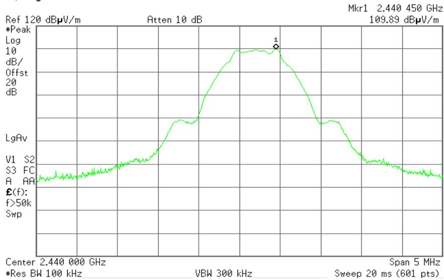
**Plot 7.2.4 Radiated emission measurements at the mid carrier frequency**
