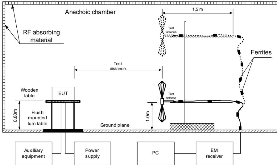
Figure 8.2.2 Setup for radiated emission measurements in 1000 – 13000 MHz range, table-top EUT
