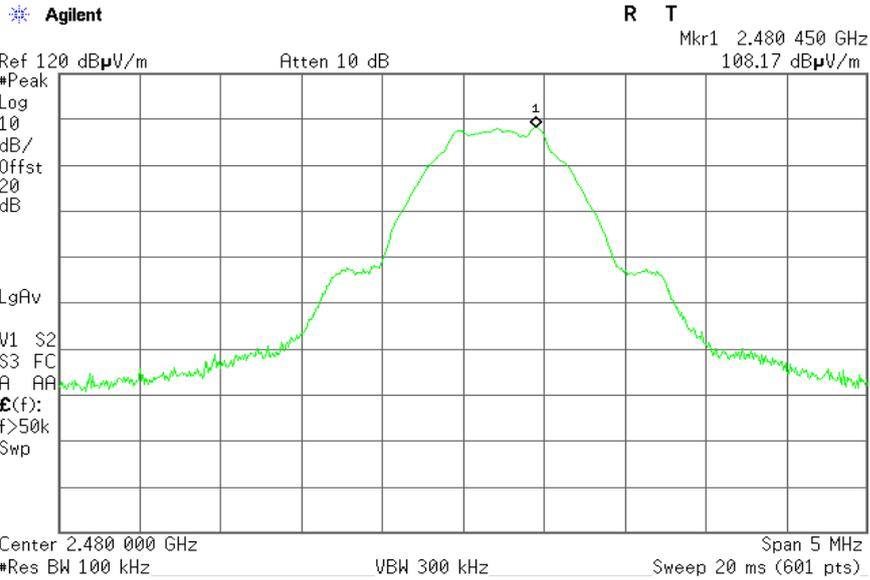
**Plot 7.2.6 Radiated emission measurements at the high carrier frequency**
