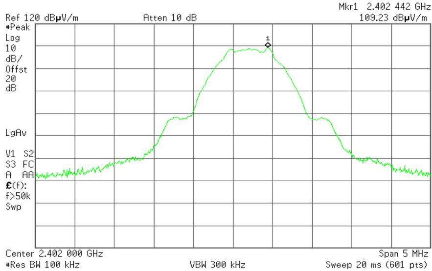
**Plot 7.2.2 Radiated emission measurements at the low carrier frequency**
