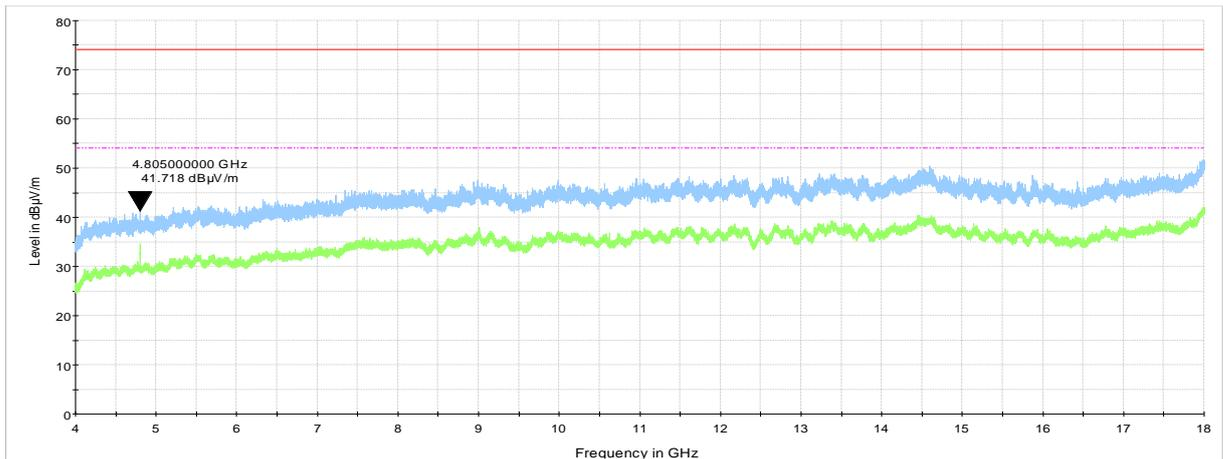
**Plot 7.2.17 Radiated emission measurements from 4 to 18 GHz at the mid carrier frequency**
