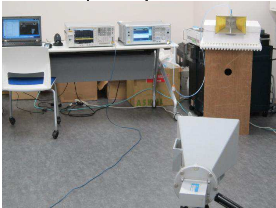
Test Setup for Generating the Radar Waveform
