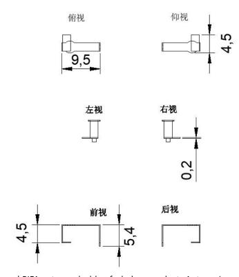
SMT on board PIFA antenna, inside of wireless products. Antenna's material is Copper-Nickel-Zinc Alloy.
