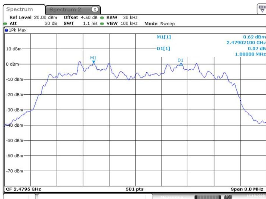
**FCC §15.247(a) (1) – 20 dB BANDWIDTH TESTING****Applicable Standard**
