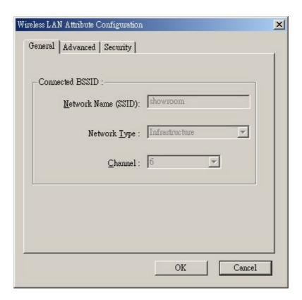
The Wireless LAN Attribute Configuration item allows you to modify the *General* information of the available network and configuration parameters for the Wireless LAN USB Card such as *Advanced* and *Security*.
