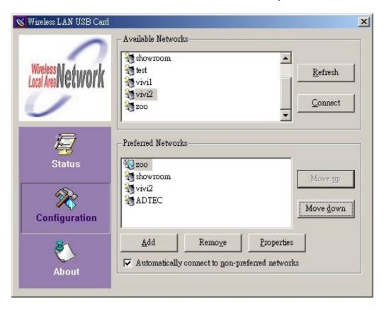
By checking **Automatically connect to non-preferred networks** check box, the Wireless LAN USB Card will automatically connect to available network even if you don't assign available network to connect or you don't have any available network in Preferred Networks at first.
