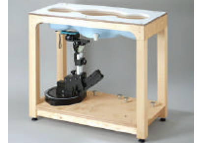
Fig. 8 Generic Twin Phantom
