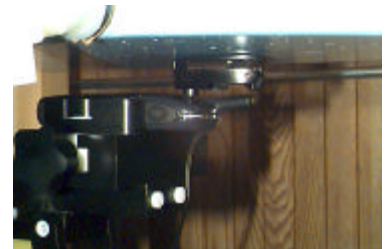
Figure 15. Body SAR Test Setup with Belt Clip
