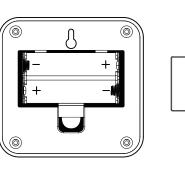
② Pay attention to the battery polarity and correctly install two new AA alkaline hatteries
