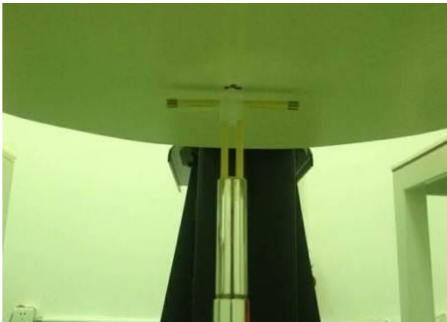
Picture 8.2 Photo of Dipole Setup
