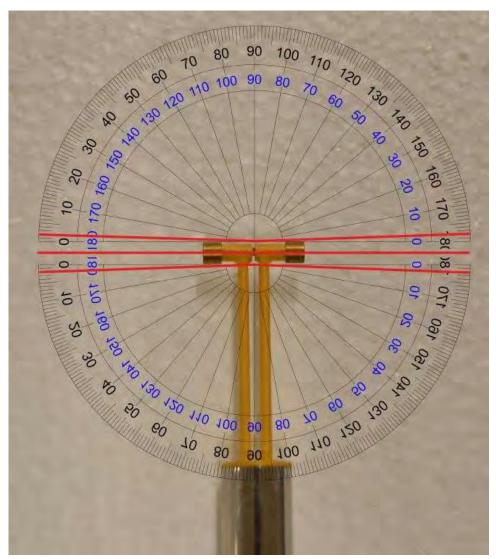
$\bullet$  The center red line indicates that the arms of the dipole fall within  $\pm 2^\circ$
