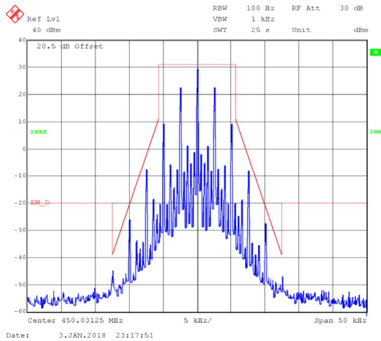
**FM,25kHz,High Power - Frequency 450.03125 MHz: 99% Occupied & 26 dB Bandwidth**
