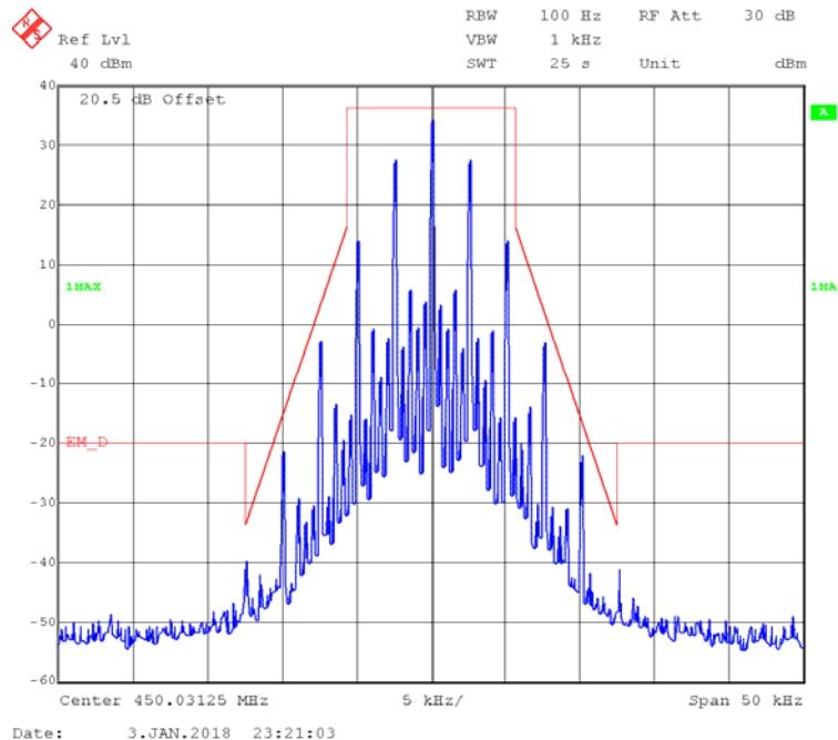
**FM,12.5kHz,Low Power - Frequency 450.03125 MHz: 99% Occupied & 26 dB Bandwidth**
