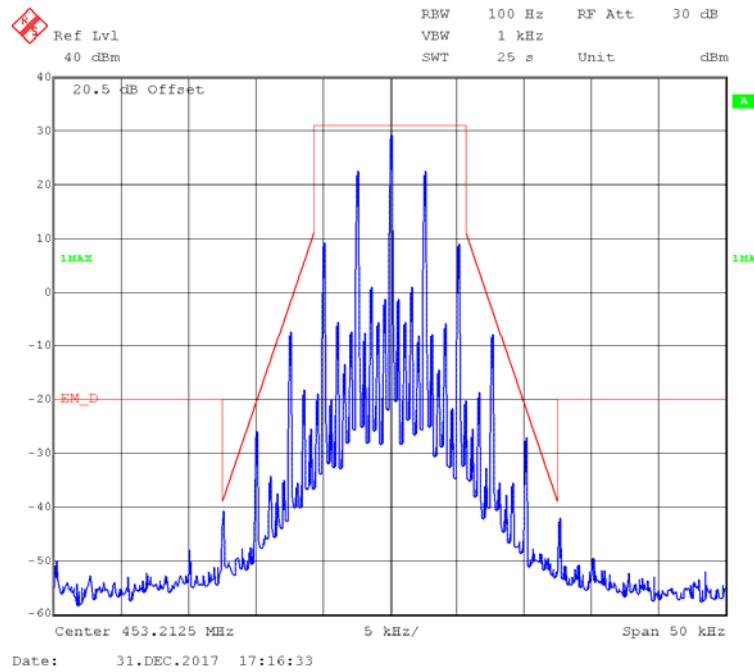
**4FSK,12.5kHz,High Power - Frequency 453.2125 MHz: 99% Occupied & 26 dB Bandwidth**
