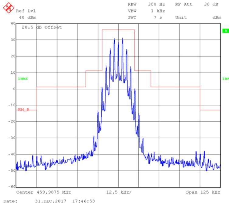
**FM,25kHz,Low Power - Frequency 459.9875 MHz MHz: 99% Occupied & 26 dB Bandwidth**
