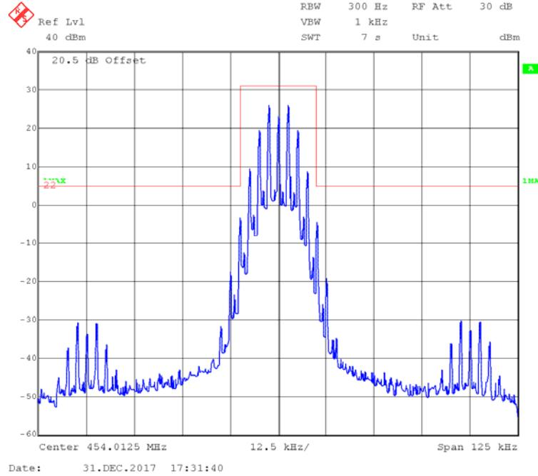
**4FSK,12.5kHz,High Power - Frequency 454.0125 MHz: 99% Occupied & 26 dB Bandwidth**
