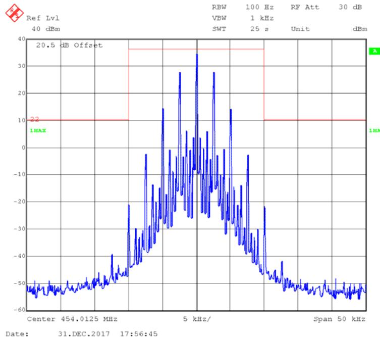
**FM,12.5kHz,Low Power - Frequency 454.0125 MHz: 99% Occupied & 26 dB Bandwidth**
