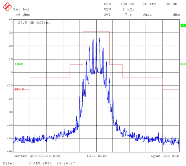
**4FSK,12.5kHz,High Power - Frequency 450.03125 MHz: 99% Occupied & 26 dB Bandwidth**
