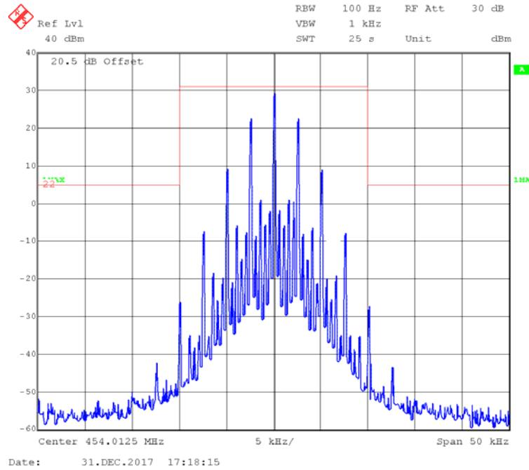
**FM,25kHz,High Power - Frequency 454.0125 MHz: 99% Occupied & 26 dB Bandwidth**
