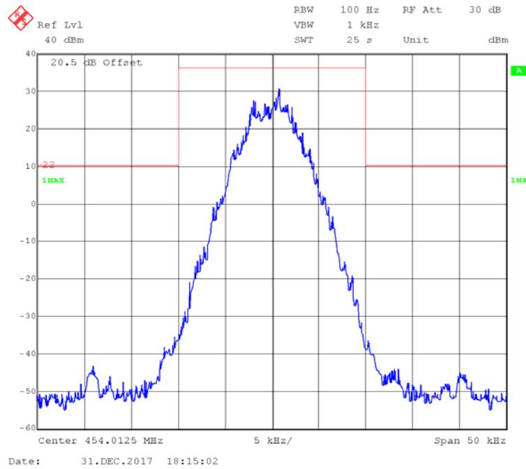
**4FSK,12.5kHz,Low Power - Frequency 454.0125 MHz: 99% Occupied & 26 dB Bandwidth**
