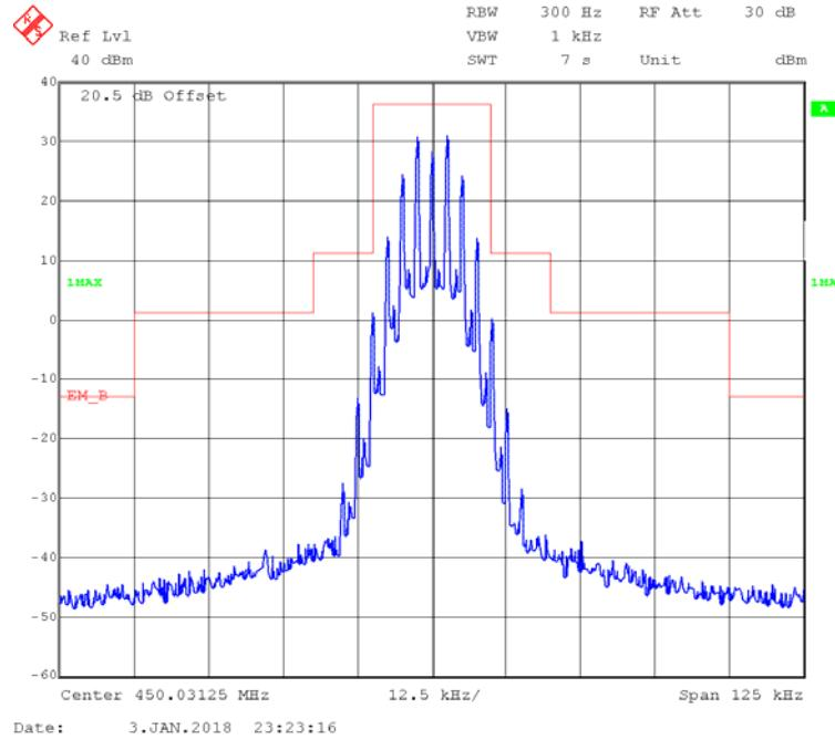
**FM,25kHz,Low Power - Frequency 450.03125 MHz: 99% Occupied & 26 dB Bandwidth**
