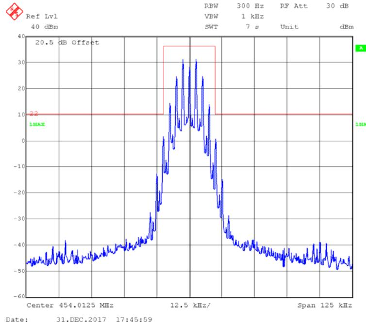
**FM,25kHz,Low Power - Frequency 454.0125 MHz: 99% Occupied & 26 dB Bandwidth**
