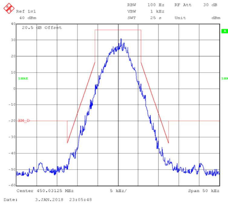
**4FSK,12.5kHz,Low Power - Frequency 450.03125 MHz: 99% Occupied & 26 dB Bandwidth**
