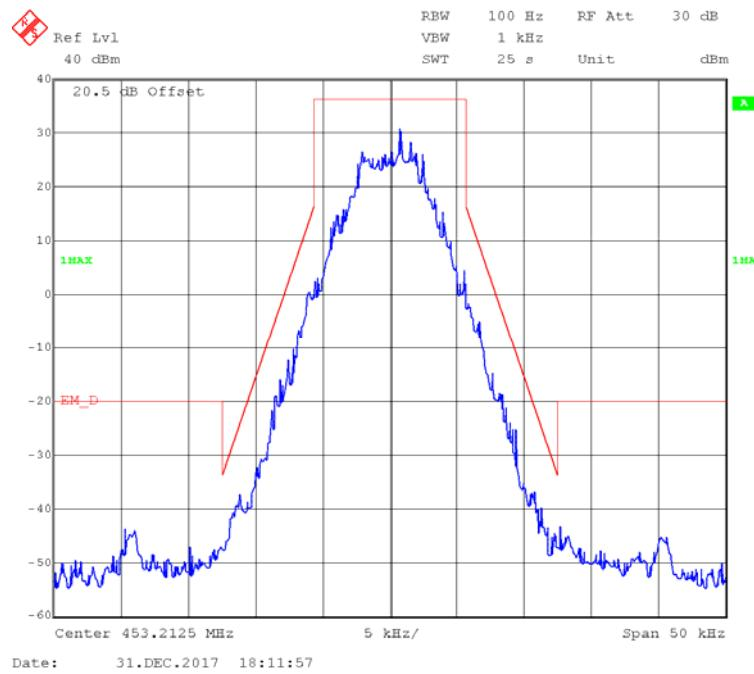
**4FSK,12.5kHz,Low Power - Frequency 453.2125 MHz: 99% Occupied & 26 dB Bandwidth**
