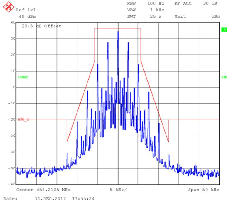
**FM,12.5kHz,Low Power - Frequency 453.2125 MHz: 99% Occupied & 26 dB Bandwidth**
