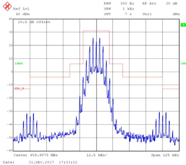
**Part 74:****FM,12.5kHz,High Power - Frequency 450.03125 MHz: 99% Occupied & 26 dB Bandwidth**
