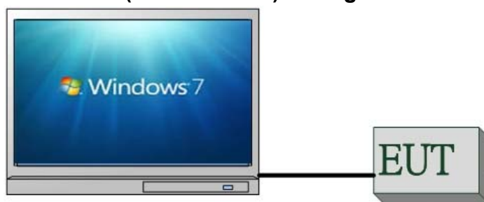
Fig. 2-2 Conducted (Antenna Port) Configuration Emission
