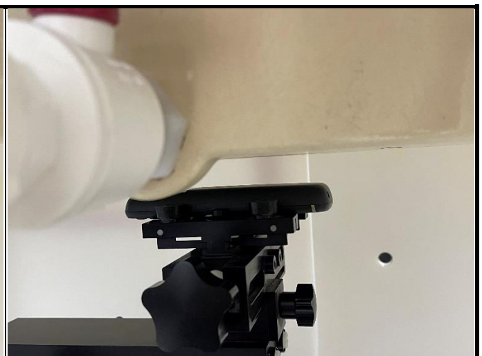
Rear Face of EUT with 1.5 cm Gap
