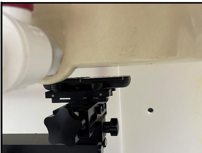
Front Face of EUT with 1.5 cm Gap
