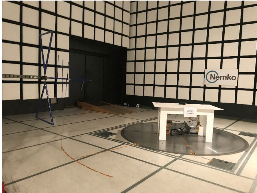
Figure 8.1.10 Radiated emissions setup from 30-1000 MHz
