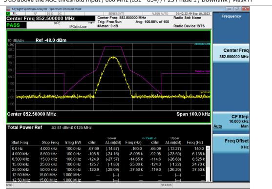
3 dB above the AGC threshold Input / 800 MHz (851 ~ 854) / P25 Phase 1 / Downlink / Mask H
