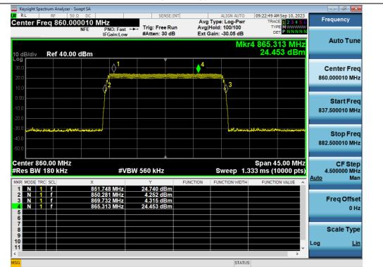
Note: The EUT only uses the frequency range of 851 MHz ~ 861 MHz.
