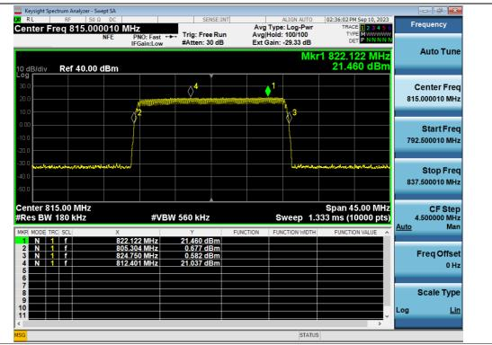
**Note:** The EUT only uses the frequency range of 806 MHz ~ 816 MHz.
