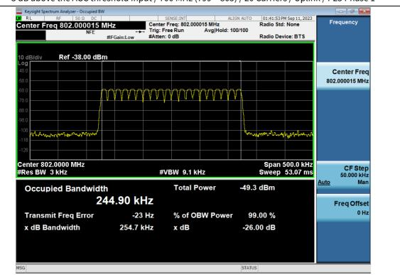
3 dB above the AGC threshold Input / 700 MHz (799 ~ 805) / 20 Carriers / Uplink / P25 Phase 1
