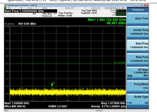
Spurious / 700 MHz (799 ~ 805) / Uplink / 20 Carriers / Additional 1559 MHz ~ 1572 MHz
