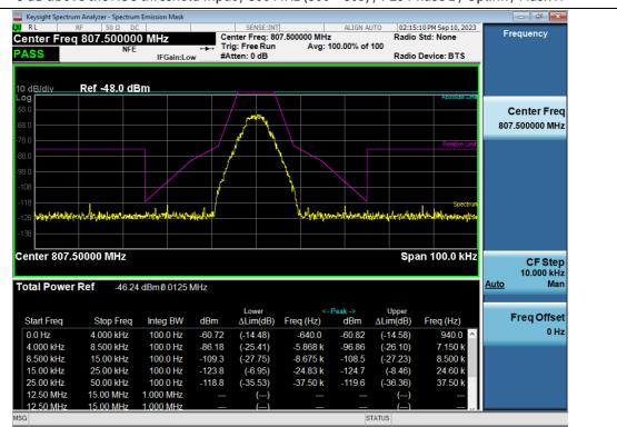
3 dB above the AGC threshold Input / 800 MHz (806 ~ 809) / P25 Phase 1 / Uplink / Mask H
