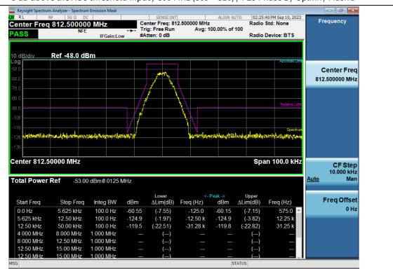
3 dB above the AGC threshold Input / 800 MHz (809 ~ 816) / P25 Phase 1 / Uplink / Mask D
