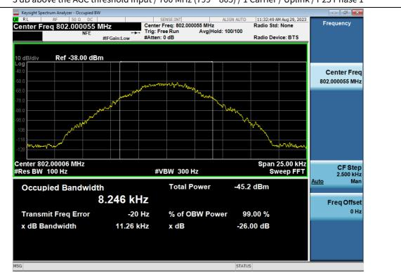
3 dB above the AGC threshold Input / 700 MHz (799 ~ 805) / 1 Carrier / Uplink / P25 Phase 1
