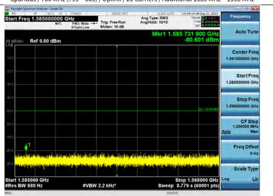
Spurious / 700 MHz (799 ~ 805) / Uplink / 20 Carriers / Additional 1585 MHz ~ 1598 MHz
