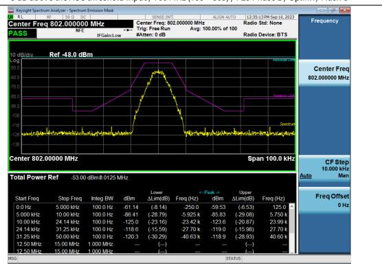
3 dB above the AGC threshold Input / 700 MHz (799 ~ 805) / P25 Phase 1 / Uplink / Mask C
