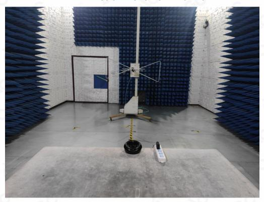
RADIATED EMISSION TEST SETUP ABOVE 1GHz
