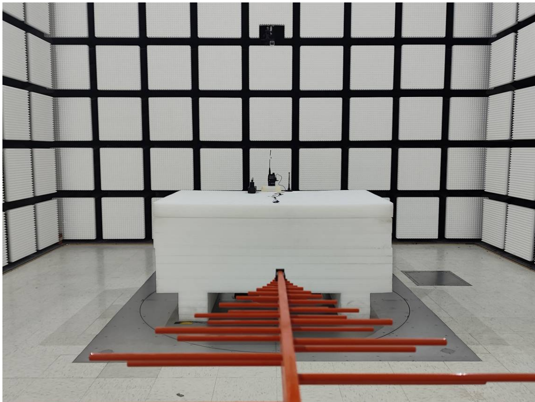
Radiated Emission Below 1GHz Rear View M2
