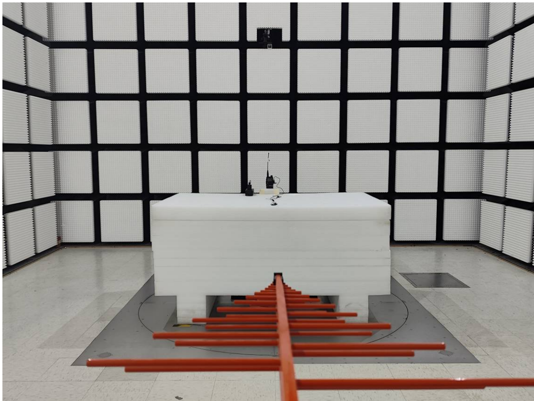
Radiated Emission Below 1GHz Rear View M1
