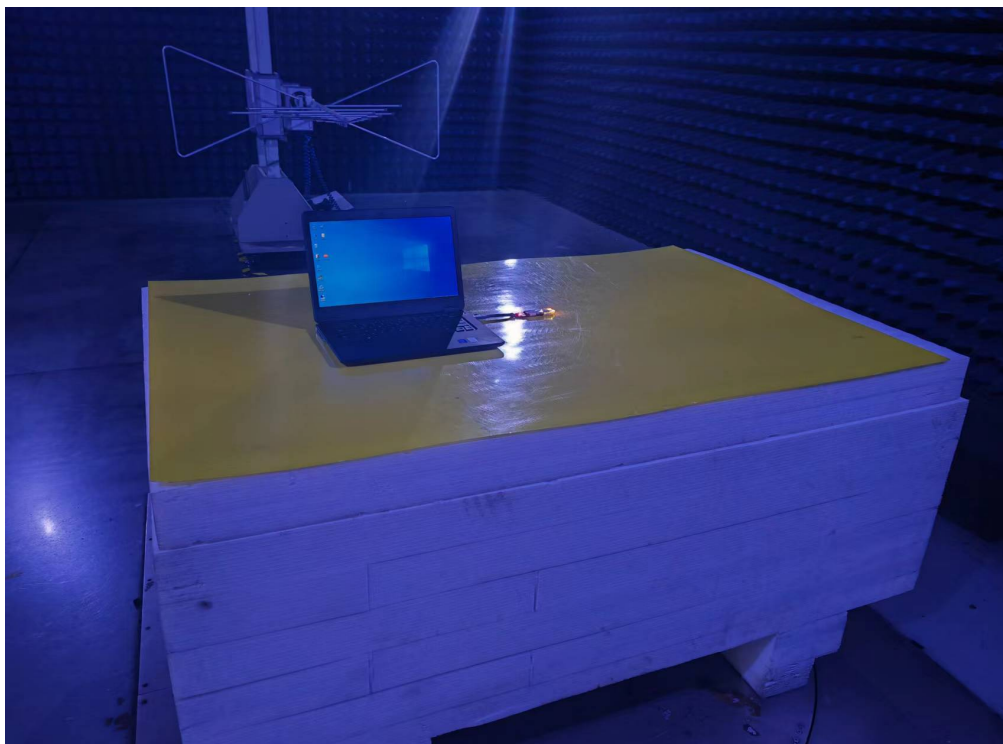
Photo of Radiated Emission Measurement (Above 1G)
