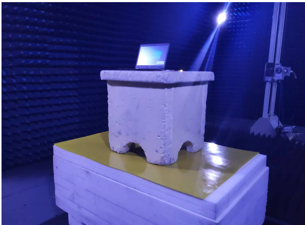
Photo of Radiated Emission Measurement (Above 1G)
