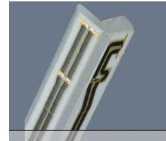
Figure 4-1 E-field Free-space Probe
