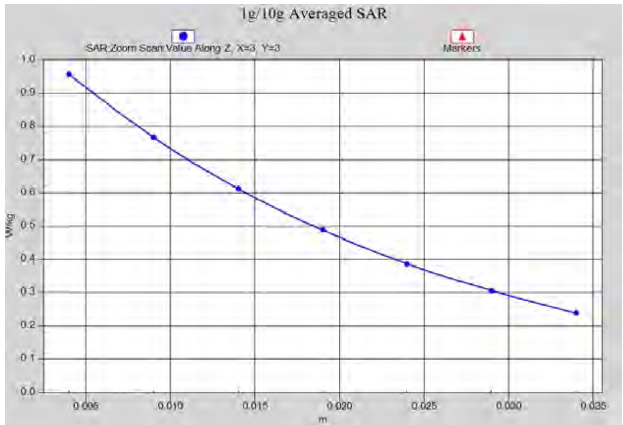
Fig. 2-1 Z-Scan at power reference point (850 MHz CH128)
