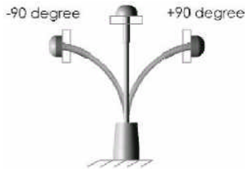
Figure 3-4: Whip bending test
