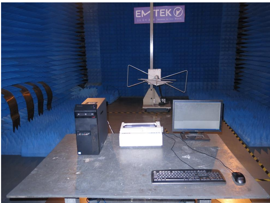
Photograph 2: Set-up for Radiated Emissions of below 1GHz
