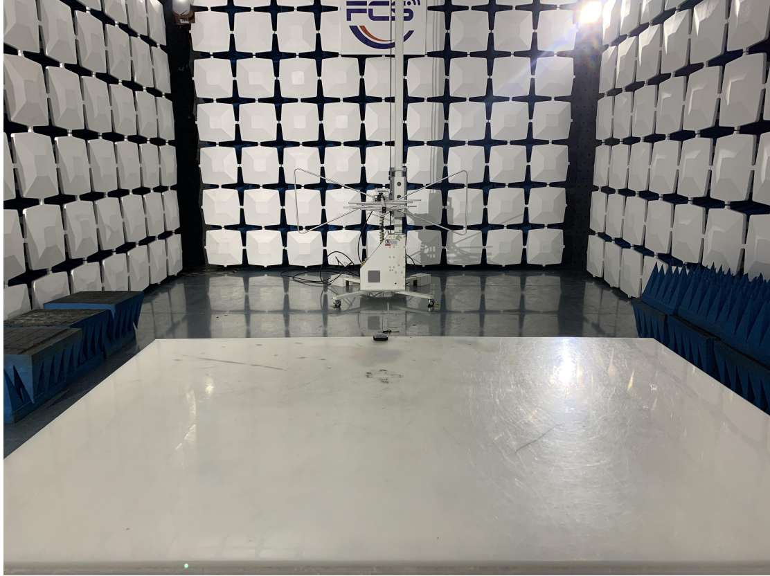
Blow 1GHz for radiated emission test setup
