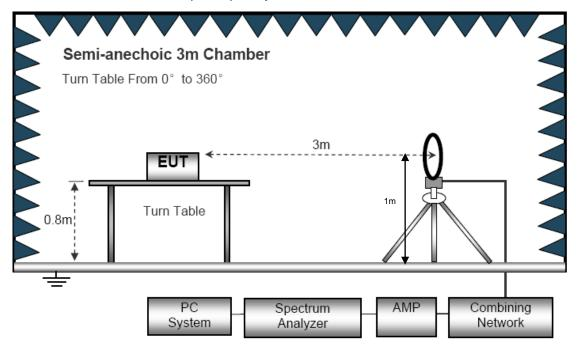
(B) Radiated Emission Test-Up Frequency 30MHz~1GHz
