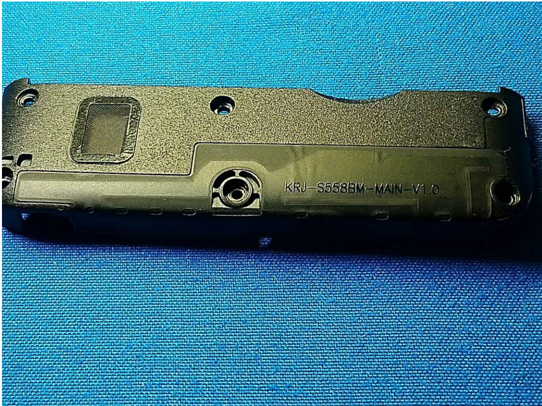
WWAN Main Antenna
