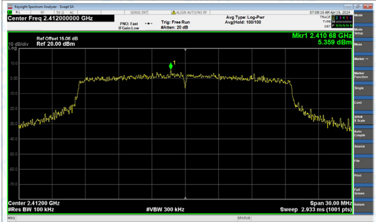
Tx. Spurious NVNT ax(VHT20) 2412MHz Ant1 Emission
