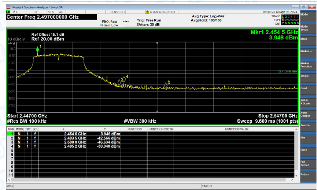
Band Edge NVNT n(HT20) 2462MHz Ant1 Emission
