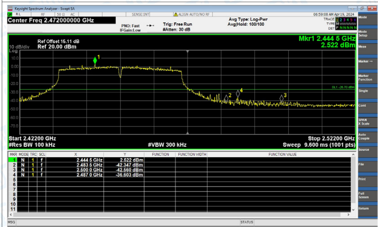
Band Edge NVNT n(HT40) 2452MHz Ant1 Emission
