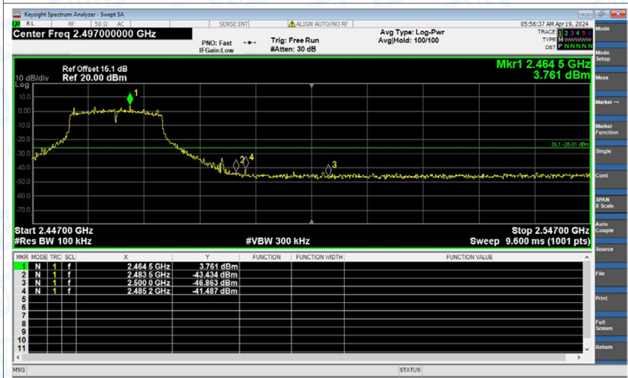
Band Edge NVNT g 2462MHz Ant1 Emission
