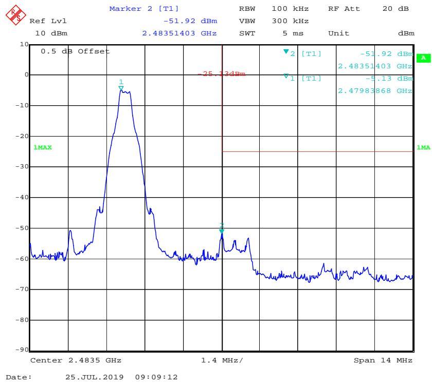
*EDR Mode ( $\pi/4$ -DQPSK):***Band Edge, Left Side**
