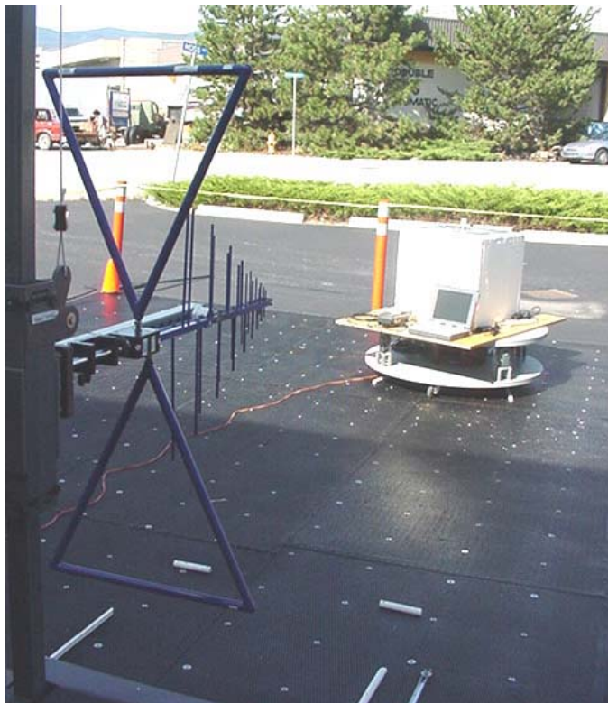
Photograph D.7-1 - BiConilog Receive Antenna with DUT Vehicle-Mount Antenna Configuration
