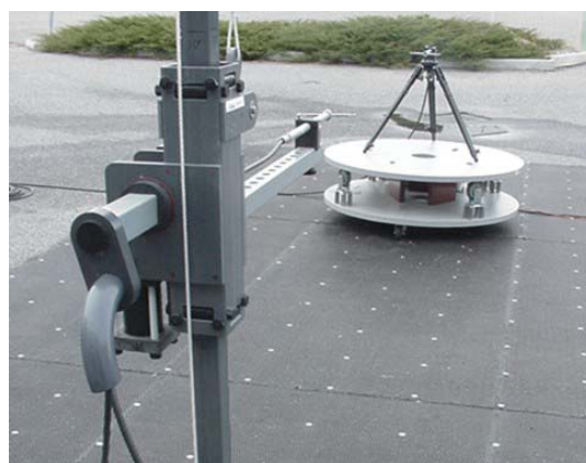
Photograph C.7-4 - Dipole Substitution Setup
