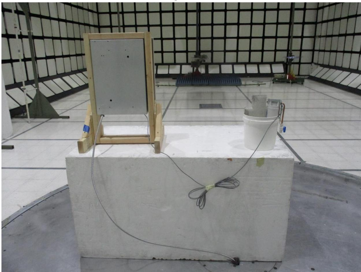
AC MAINS LINE CONDUCTED EMISSION Configuration 1
