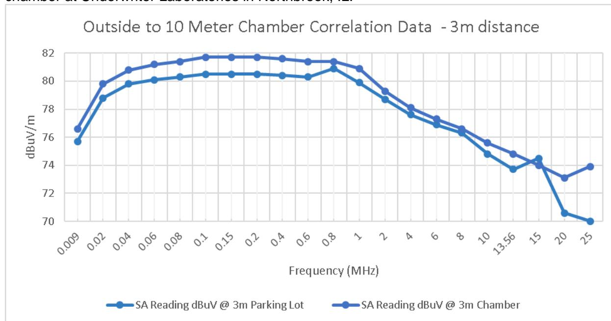
Correlation measurements were conducted using a signal source with an antenna outside in open area (parking lot). Immediately following the measurements the same setup was moved inside the 10 meter semi-anechoic chamber and the measurements were repeated. The above plot shows the difference in levels measured between outside and the 10 meter semi anechoic chamber.
