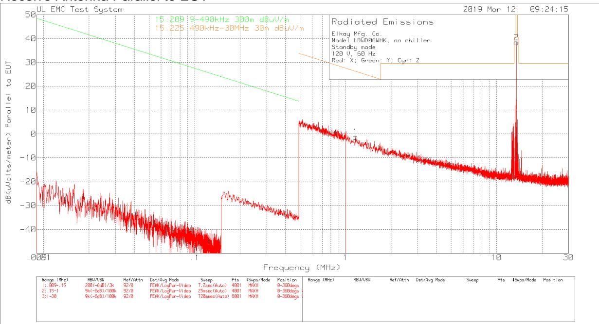
RE 9kHz-30MHz 3m E-Field Loop 3 axis with CorrectDistances FCC 15.225 ESCI.TST
