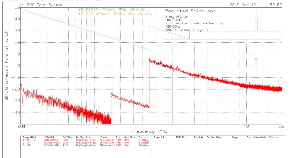
RE 9kHz-30MHz 3m E-Field Loop 3 axis with CorrectDistances FCC 15.225 ESCI.TST
