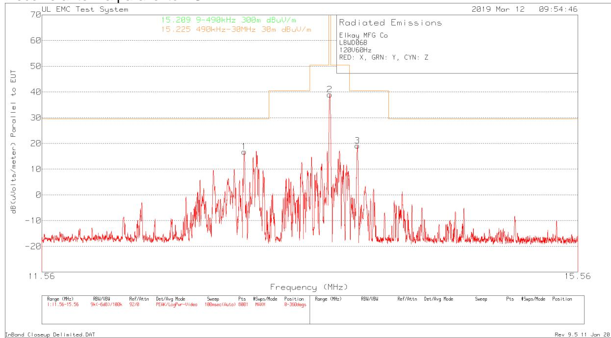
Receive Antenna Perpendicular to EUT
