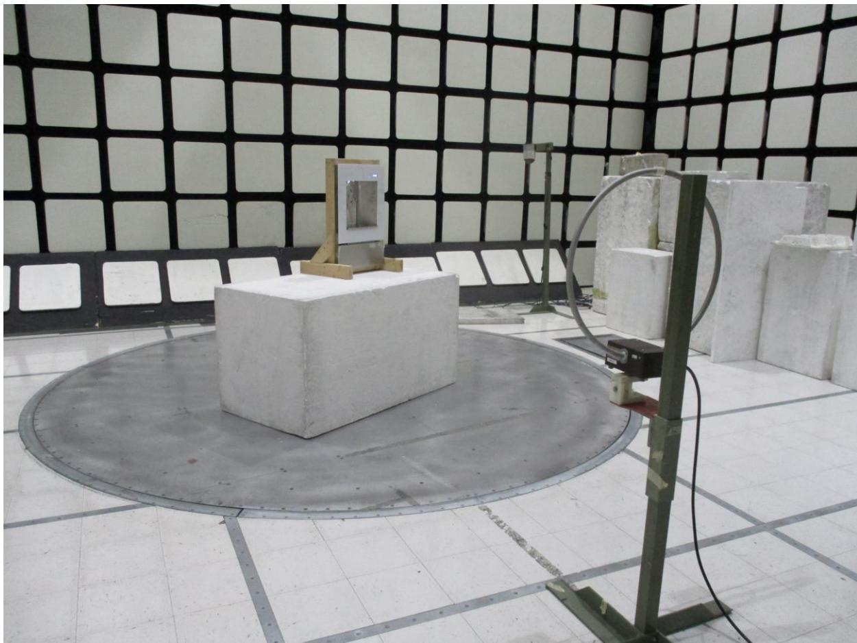
**RADIATED EMISSION BELOW 30 MHz for Configuration 2**
