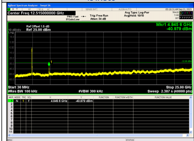
Spurious Emission IEEE 802.11ax_Channel 3_40MHz_Antenna 0_RU&Index 484RU65
