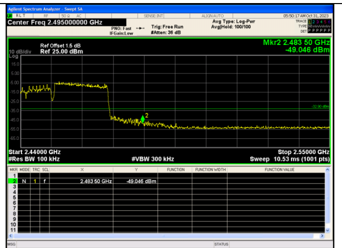
Out Of Band Emission IEEE 802.11ax_Channel 9_40MHz_Antenna 0_RU&Index 242RU62
