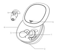
1.Pilot lamp 2.Battery indicator 3.Function operation keys 4.Type-Ccharging port 5.Headphone charging contact 6.Earphone opening
