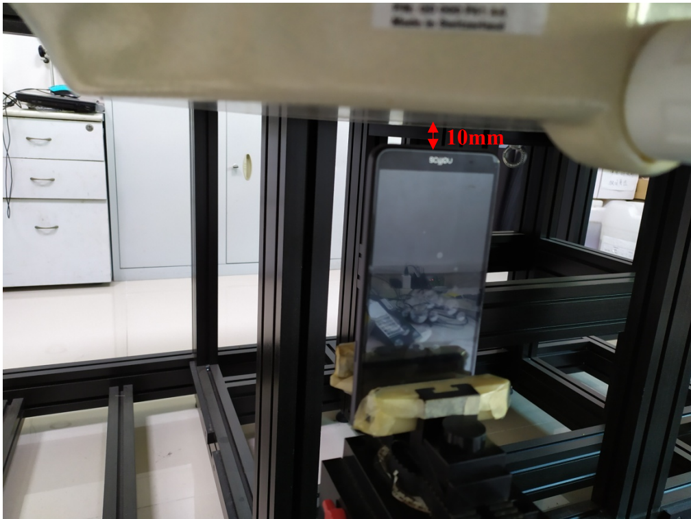
Body Bottom Setup Photo (10mm)
