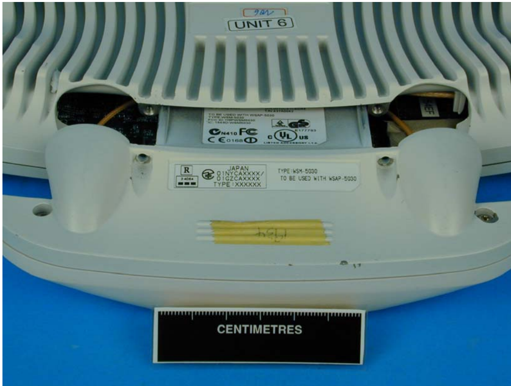
WSM5030 2.4GHz Integral Antenna Outside Case Rear Showing Connection to WSAP5030
