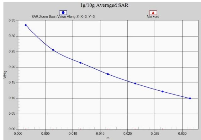
Z-Scan at power reference point (GSM850)
