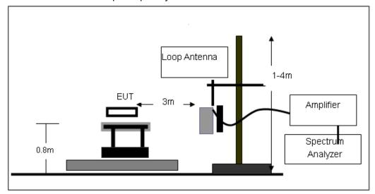
(B) Radiated Emission Test-Up Frequency 30MHz~1GHz
