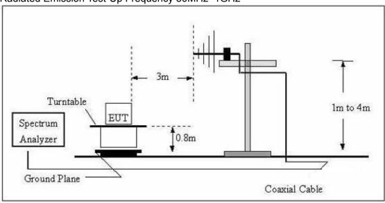
(C) Radiated Emission Test-Up Frequency Above 1GHz
