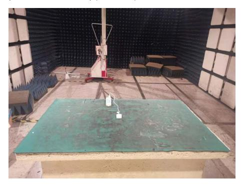
Spurious Emission Test Setup (Above 1GHz)
