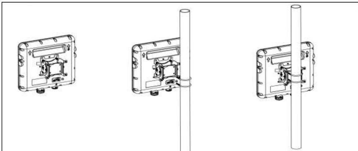
Figure 6-1-2-1 To mount the CPE to wall
