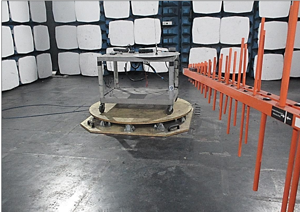
Figure 12 - Test Setup - 30 MHz to 1 GHz
