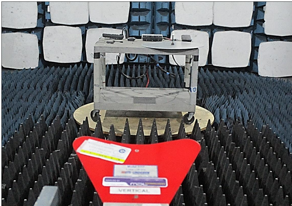
Figure 13 - Test Setup - 1 GHz to 13 GHz
