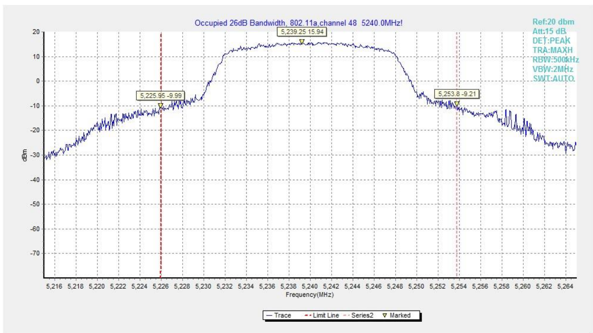
Fig.3 Occupied 26dB Bandwidth (802.11a, 5240MHz)
