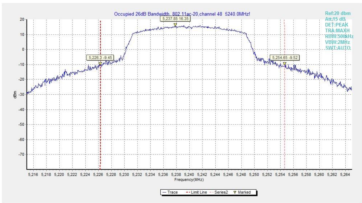
Fig.13 Occupied 26dB Bandwidth (802.11ac-HT20, 5240MHz)
