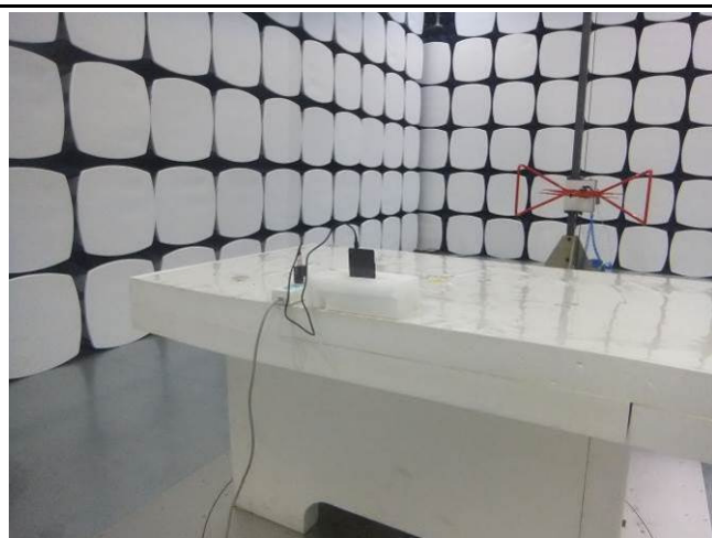
Conducted Emissions Test Setup Front View
