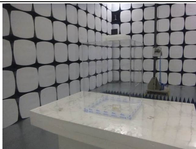
Radiated Spurious Emissions Test Setup Above 1GHz
