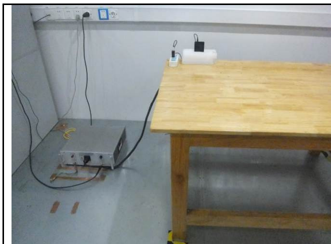
Conducted Emissions Test Setup Front View
