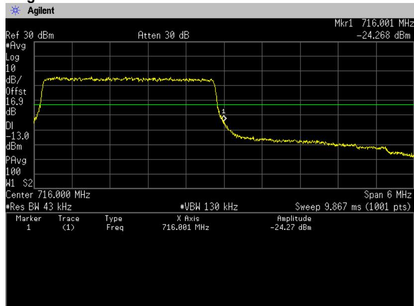
**16QAM, BW 3MHz, RB1-0****Channel: Low**
