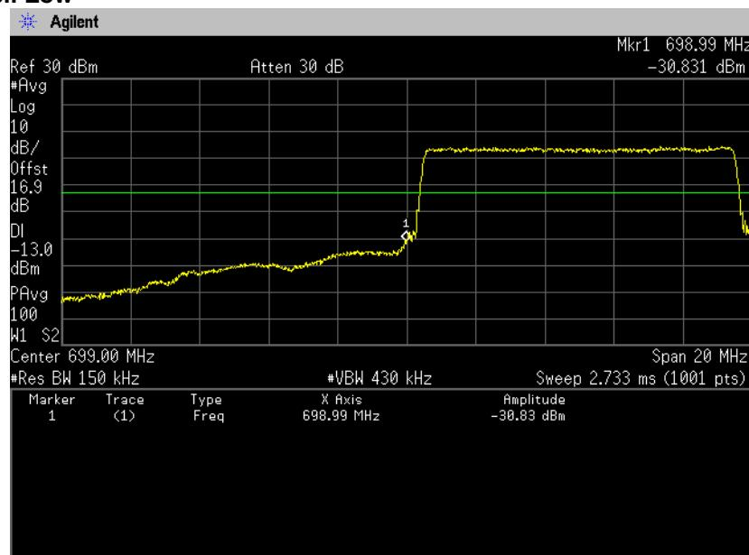
**16QAM, BW 10MHz, RB50-0****Channel: High**
