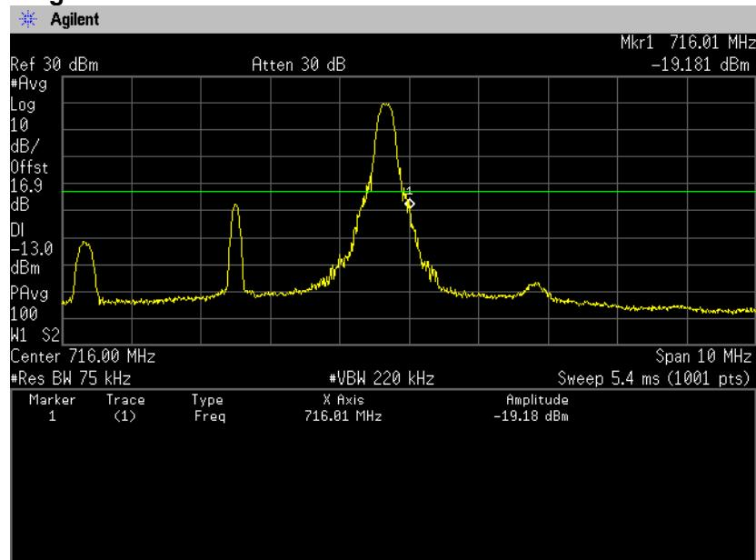
**QPSK, BW 5MHz, RB25-0****Channel: Low**
