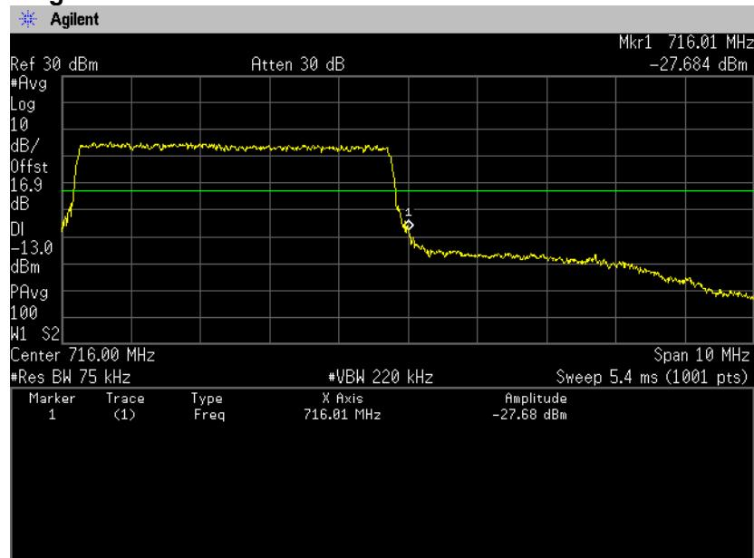
**QPSK, BW 10MHz, RB1-0****Channel: Low**
