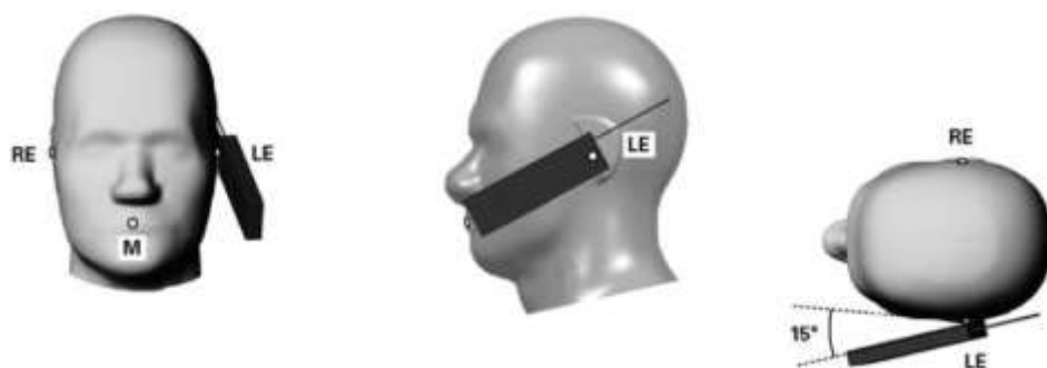
Figure 8.5. Tilt 15° position of the wireless device
