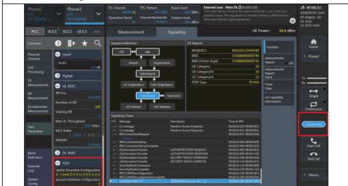
Call 3:Select PCC Configuration for LTE TDD " Uplink Downlink Configuration" set to "0" And then Select "connect" button.
