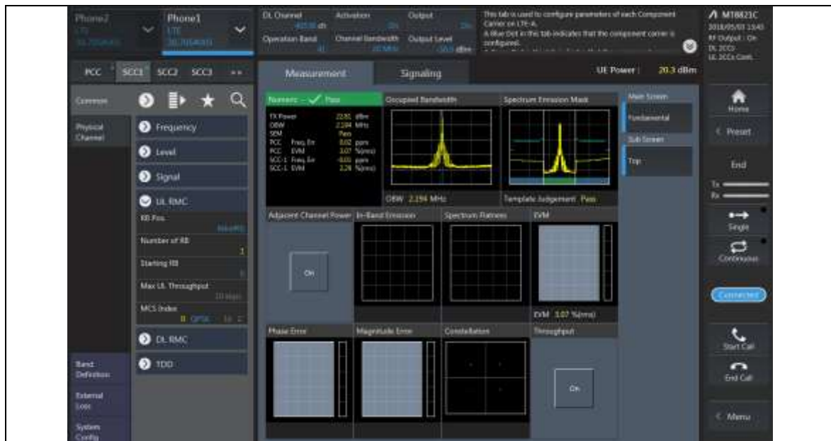
Call 4: Set to RB, offset, BW, modulation of SCC channel.
