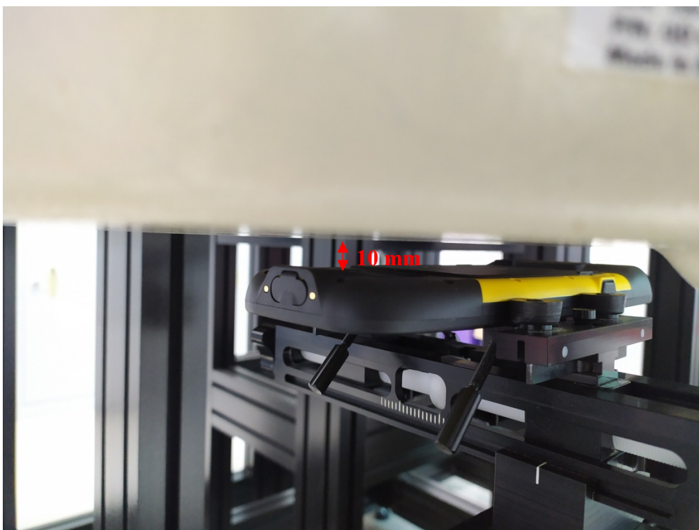
Body (Worn) Back Setup Photo (10mm)
