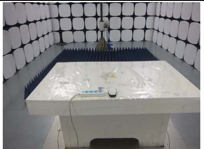
Radiated Emissions Test Setup Above 1GHz - Side View
