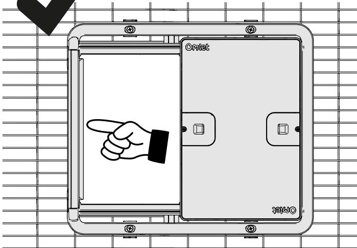
The safety sensor bar which detects if an object is blocking the door from closing will only work properly if the door is installed correctly. In the image to the left the opening of the coop is smaller than the opening of the Autodoor. In this case the Autodoor's safety sensor bar might not operate correctly. To solve this move the Autodoor so that the opening is set back from the edge of the safety bar by at least 0.2 in (5 mm) like in the picture to the right...
