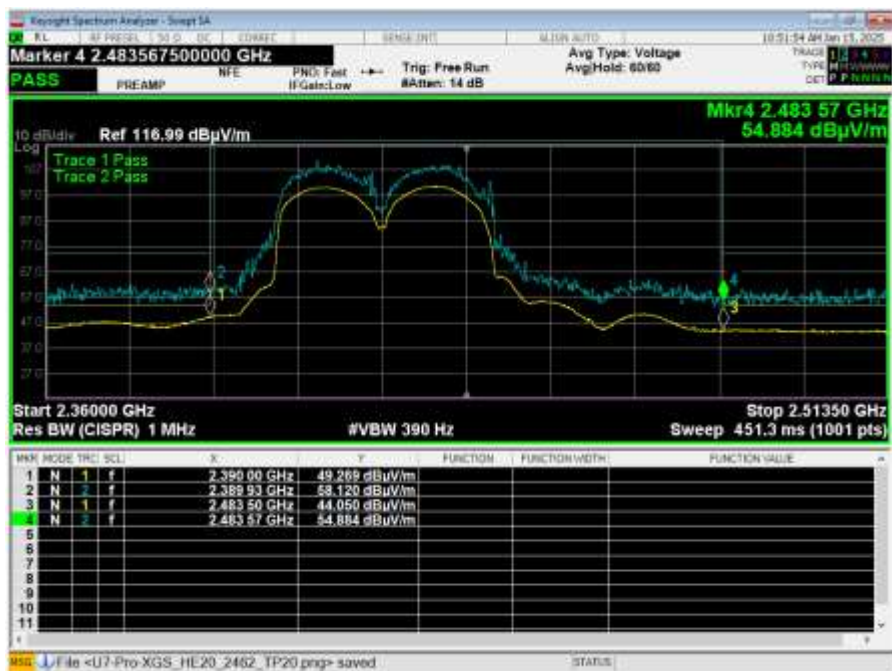
Graph 18: Lower Band Edge Plot – 2422 MHz – ax40 Mode
