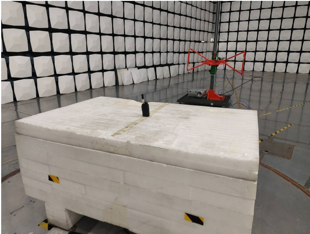
Radiated Emission Above 1GHz View
